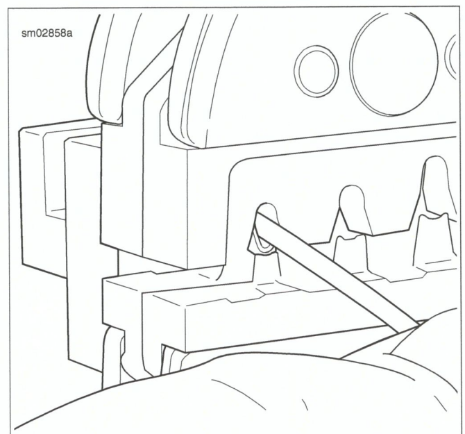
Figure A-22. Stripped Lead at Up Angle
